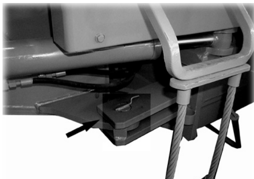
17. Articulation lock pin (apply grease)
